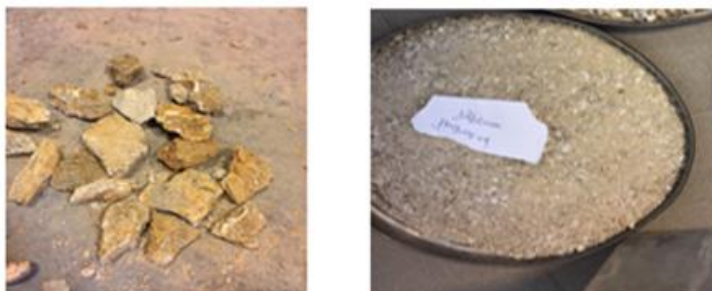
Plate 1: Samples of the Warake (left) and Spain-imported Gypsum (SIG Right) used for the study
